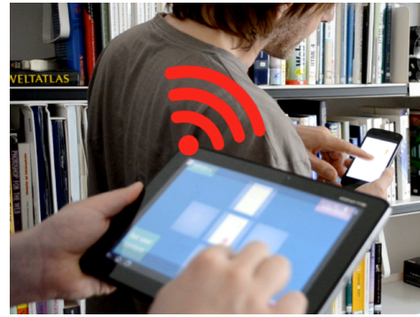
Figure 1. The participant's mobile phone (background) and the tablet computer of the Wizard (foreground) are paired wirelessly. Input of the participant is displayed on the Wizard's device (‘live-view’), where the Wizard can react to it remotely.
